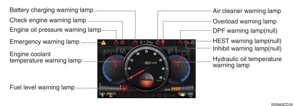
Each warning lamp on the top of the LCD pops up on the center of LCD and the buzzer sounds when the each warning is happened. The pop-up warning lamp moves to the original position and blinks when the select switch is pushed. And the buzzer stops. Refer to page 3-11 for the select switch.
