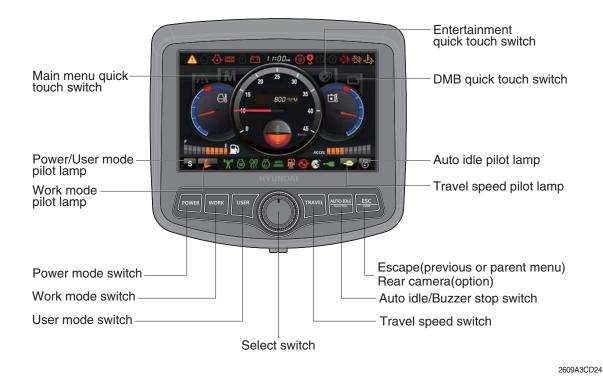
When the switches are selected, the pilot lamps are displayed on the LCD. Refer to the page 3-7 for details.
