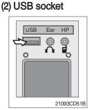
① This socket is used to charging the mobile phone.
